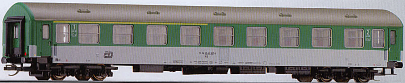
Reisezugwagen 1./2. Klasse, Typ Y/B 70, der ČD 1st/2nd class passenger coach, type Y/B 70, of the ČD
