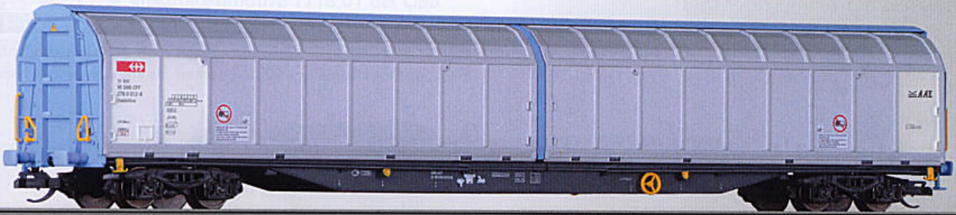
Schiebewandwagen Habbis 345 der SBB Sliding cover box car Habbis 345 of the SBB
