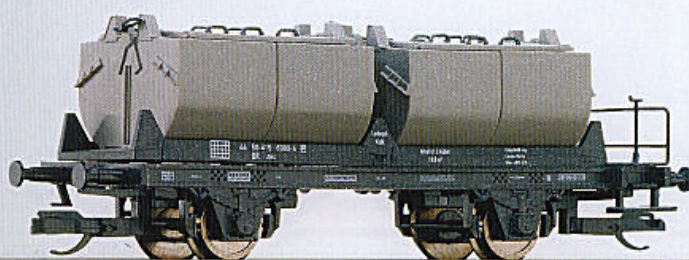
Kalkkübelwagen Lbks der DR Skip car for transport of limestone of the DR
