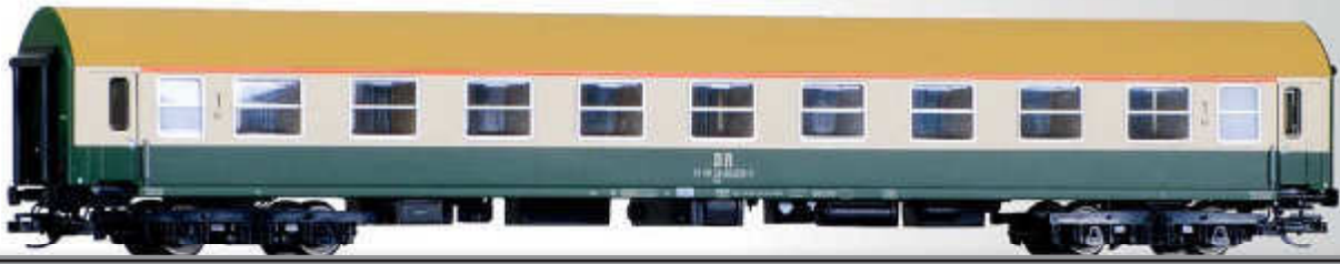
Reisezugwagen 1. Klasse, Typ Y/B 70, der DR 1st class passenger coach type Y/B 70 of the DR
