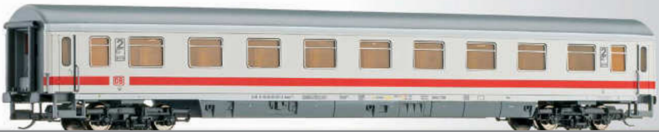
Reisezugwagen 2. Klasse, Bvmz 111.2 der DB AG 2nd class passenger coach, Bvmz 111.2 of the DB AG
