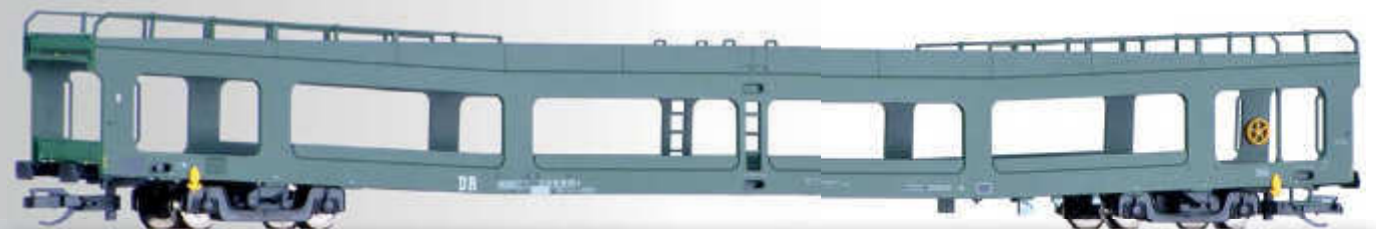
Autotransportwagen DDm der DR Car DDm of the DR for automobile transport
