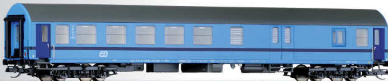
Sitz-/Gepäckwagen 2. Klasse, Typ Y/B 70, der ČD 2nd class passenger coach with baggage compartment, type Y/B 70, of the ČD
