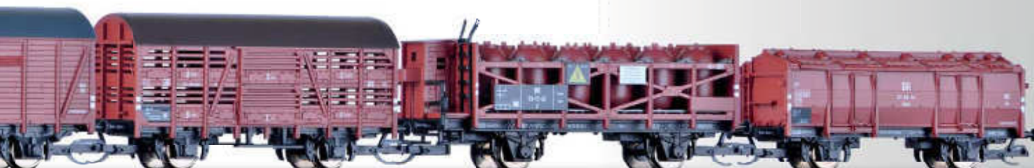
Freight car set of the DR with six different freight cars (low side car Xu, open car Omu, box car Glxu, partition car for animal transport V, acid pot car Z, hinged cover car Kmm)
