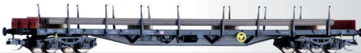
Rungenwagen Rs-u 659 der DB AG, beladen mit Schienen Stake car Rs-u 659 of the DB AG loaded with tracks
