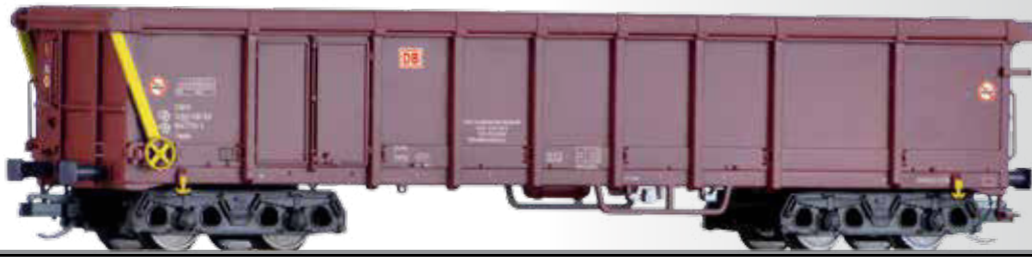
Rolldachwagen Taems der DB AG Sliding roof car Taems of the DB AG
