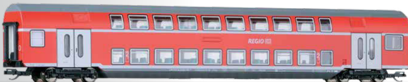
Doppelstockwagen 2. Klasse DBz 750 der DB AG 2nd class double-deck coach DBz 750 of the DB AG
