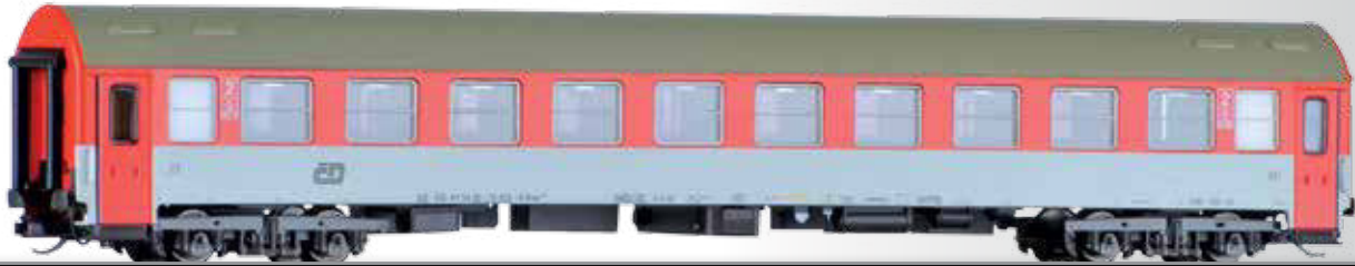
Reisezugwagen 2. Klasse Bee, Typ Y/B 70, der ČD 2nd class passenger coach Bee, type Y/B 70, of the ČD
