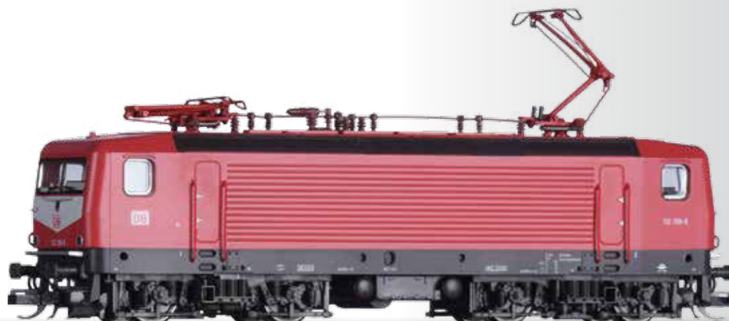
Elektrolokomotive BR 112.1 der DB AG Electric locomotive class 112.1 of the DB AG
