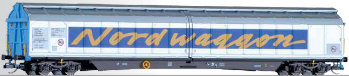
Schiebewandwagen Habiins der Nordwaggon Sliding cover box car Habiins of the Nordwaggon
