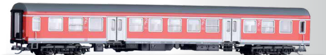
Reisezugwagen 2. Klasse By 439, Bauart Halberstadt, der DB AG 2nd class passenger coach By 439, type Halberstadt, of the DB AG
